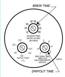
Fig. 15 Adjust BrewTime and Dripout Time
