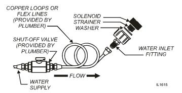
Fig. 2 Water Supply Installation
