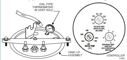
Fig. 14 Checking and Adjusting Brew Temperature
