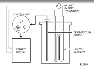
Fig. 5 Heat Control Diagram
