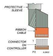
Fig. 20 Keypad Ribbon Cable Hook-Up
