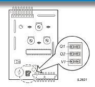
Fig. 19 Controller Jumpers
