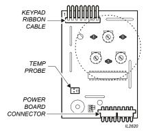
Fig. 18 Controller Hook-Up
