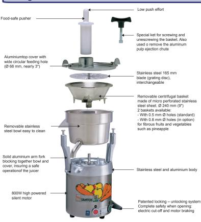
For all fruits and vegetables (citrus fruits must be peeled). Continuous juice production by centrifugal action and automatic pulp ejection.
