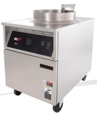
This extra-large electric auto-lift fryer is designed for simple operation, long life, and high product volume. The manual controls are easy to use and the lower initial cost will get you cooking fast. The BKI® BLF-F fryer cooks up to 18 lb (8.2 kg) of product in one cycle and holds 75 lb (34 kg) of oil.
