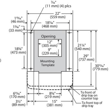
Recommended counter opening size 9" (229 mm) x 12" (305 mm) for utilities and tubing. Opening can be located anywhere within the shaded area.
