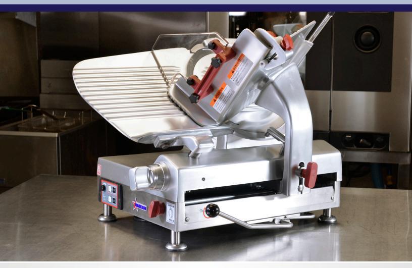
Omcan's MS-IT-0330-N is equipped with automatic sliding carriage and two independent high performance fan cooled motors: one for the carriage and one for the blade. The gears are constantly bathed in oil. The polished anodized aluminium body along with its high carbon, hard chromed blade provides long life and durability. Easy to disassemble and clean.
